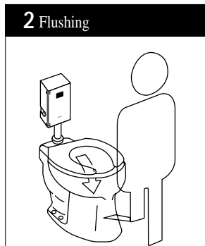
After using over 4 seconds, when a user leaves the fixture, the sensor automatically sends a signal to the operating unit to activate the flush valve.
