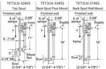
Depending on X, the frame may not be centered to Supply G as shown. \*Leave some room for elbow nut from the wall for future maintenance.
