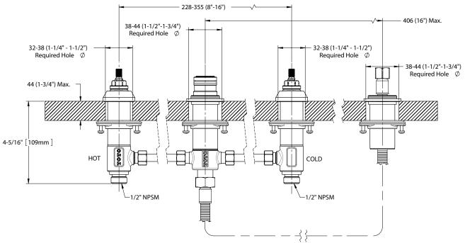
Important Note: This product must be installed after the deck or tub rim is finished.
