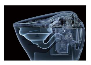
integrated WASHLET personal cleansing system with warm, aerated water to cleanse, warm air dryer, heated seat, and in-bowl catalytic deodorizer; and energy- and water-saving features.
