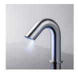
The Standard-R TOUCHLESS Faucet offers TOTO's proprietary EWATER+ technology. This unique smart-sensor faucet automatically mists the lavatory with electrolyzed water, a well-known cleaning agent, which reduces the need for harsh cleaning chemicals. EWATER+ is produced from ordinary tap water by electrolyzing its chloride ions. It is completely free of added chemicals, detergents, or harsh cleaning agents. Over time, EWATER+ returns to its original state as ordinary tap water.
