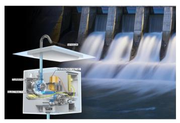
ECOPOWER technology harnesses the energy of running water to power the TOTO smart-sensor faucet and flush valve's electronics (no need for hard-wiring to the building's electrical system or for routine battery replacement).
