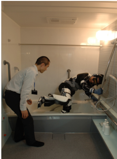
Wearing an Age Simulation Suit, a TOTO Product Engineer learns first hand the difficulty a physically challenged person has getting out of the tub.
