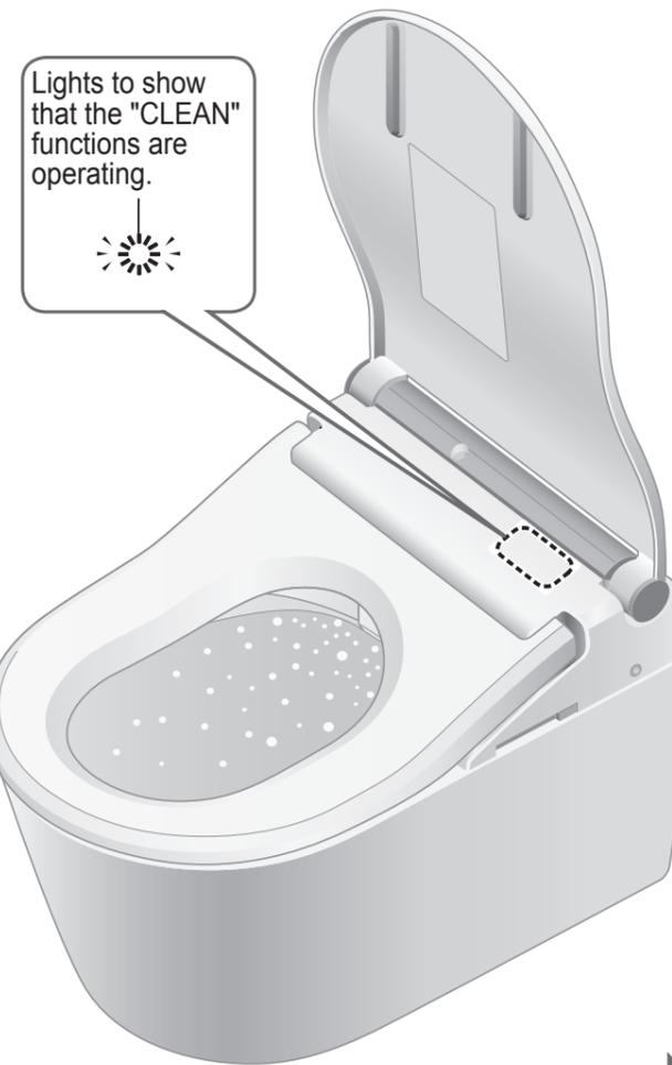
The self-cleaning functions operate automatically.
