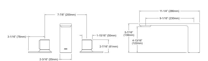
IMPORTANT NOTE: This valve/trim can only be installed in a built-up deck. It cannot be installed on pre-finished deck or on tub rim.
