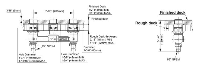
IMPORTANT NOTE: This valve/trim can only be installed in a built-up deck. It cannot be installed on pre-finished deck or on tub rim.
