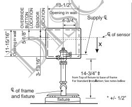
Always position the sensor above upright toilet seats and grab bars X,  $\ddagger$  = At least 5" clearance from sensor to tip of toilet seat up position or to top of grab bar is required to avoid false detection.
