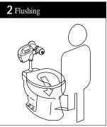
After using over 5 seconds, when a user leaves the fixture, the sensor automatically sends a signal to the operating unit to activate the flush valve.
