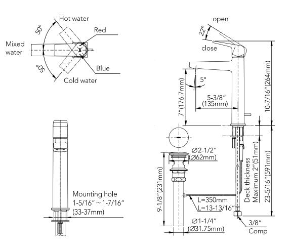
NOTE: The above dimensional unit is inch. The dimension in ( ) is reference mm.
