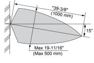
X", ‡ = At least 5" clearance from sensor to tip of toilet seat up position or to top of grab bar is required to avoid false detection.
