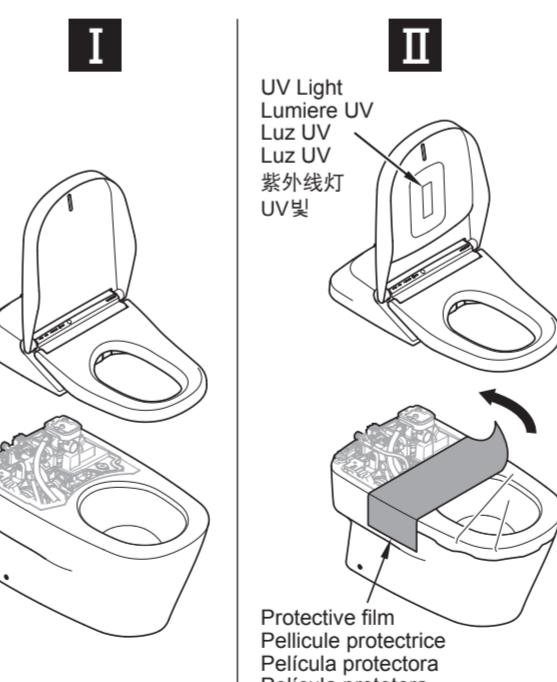
Be sure to remove the blue protective film before mounting the functional unit.
